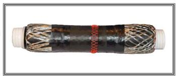
The CSJA cold shrinkable joint for 15 kV through 35 kV is designed to splice tape shield, wire shield, LC shield, UniShield, JCN and flat strap shielded cables.
